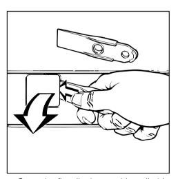
■ Open the flap (in the machine plinth).
